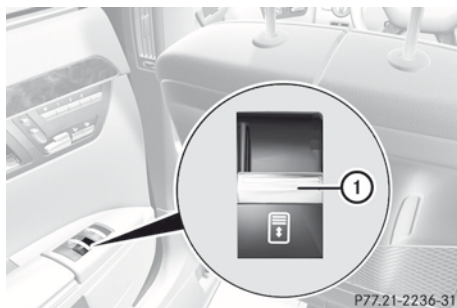
Door control panel in rear
