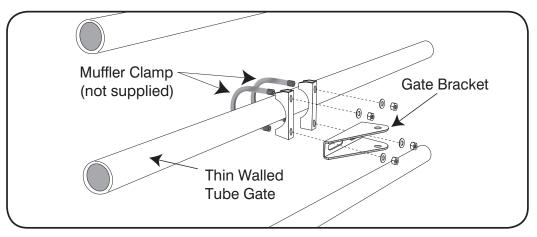
Muffler Clamp for Gate Bracket
