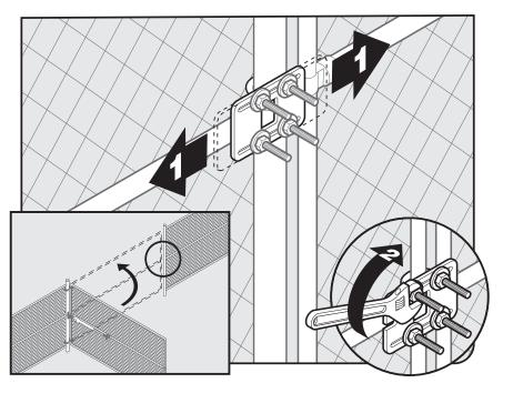
**Note:** For MM572W installations, the closed position stop plate should be installed on the leading edge of the PRIMARY gate leaf, and adjusted to close against the leading edge of the SECONDARY gate leaf.
