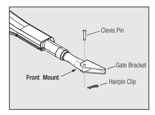
**NOTE:** Substitute a **Pin Lock** for the clevis pin on the front mount of the gate operator to prevent theft of the operator from the gate (*see accessory pages in back of this book*).
