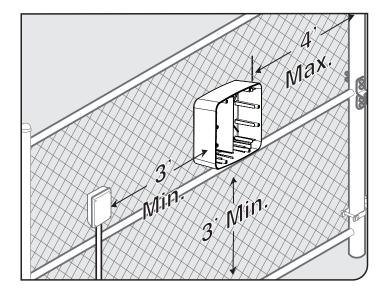
Identify a suitable mounting location for your control box at least 3 ft. from the ground and no more than 4 ft. from the primary operator.
