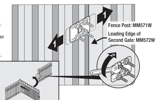
**Note:** For MM572W installations, the closed position stop plate should be installed on the leading edge of the PRIMARY gate leaf, and adjusted to close against the leading edge of the SECONDARY gate leaf.
