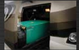
All Berkshire's come equipped with a 6.0KW generator on a slide tray.
