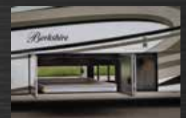
Standard cafe compartment doors with pass thru storage and optional slide-out storage tray.
