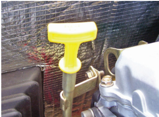
Figure 4.3 — Oil Dipstick and Fill, 12, 14, 16, 17 & 20kW
