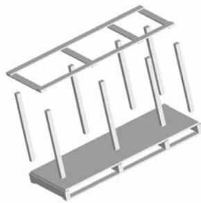
Internal packaging structure with cardboard walls;
