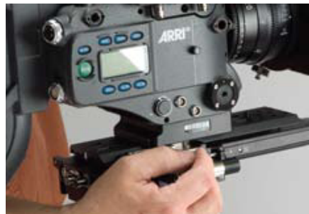
Closing the locking lever.
