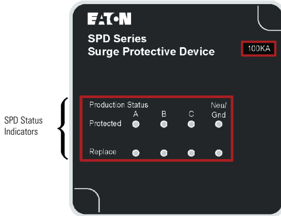
Figure 6-7. Status Indicator Display for Non-EMS monitored SPD
