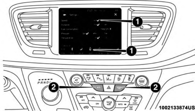
Uconnect 4C/4C NAV Buttons On The Touchscreen And Buttons On The Faceplate
