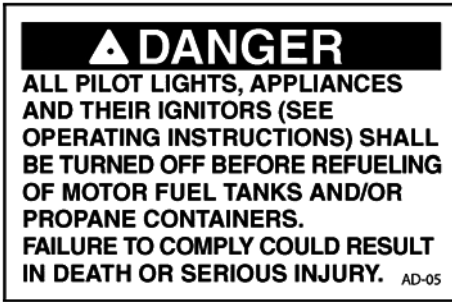
Fig. 7.9 Refueling warning label
