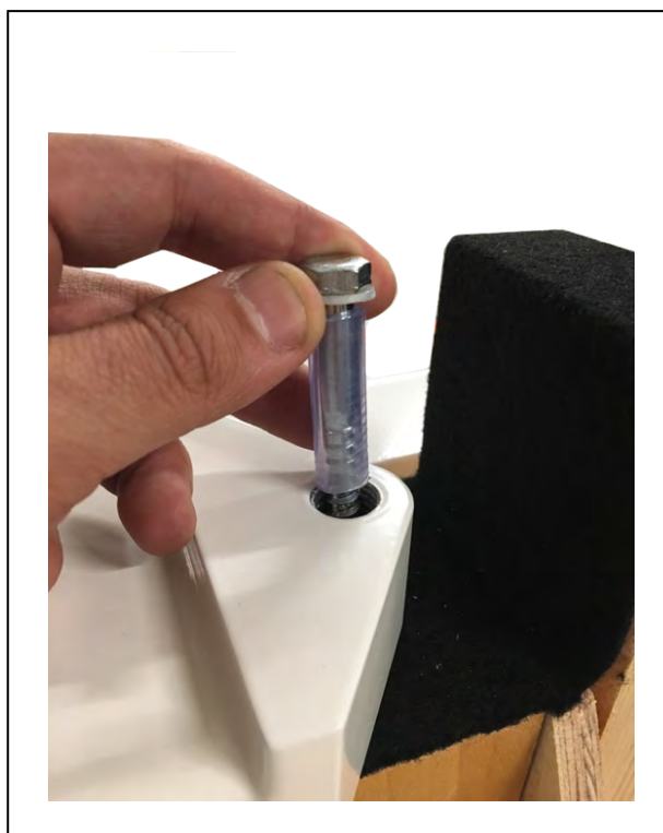
Figure 9-3. Removal of Bolt
