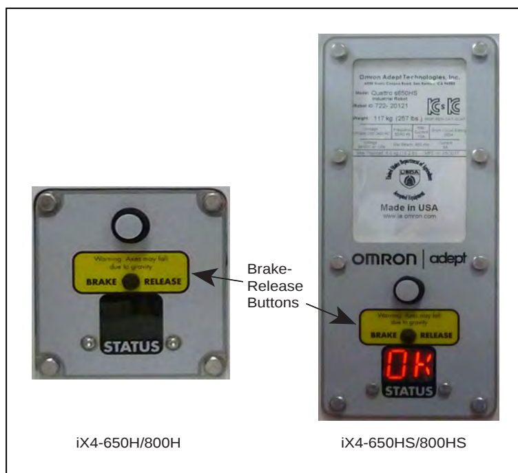
Figure 5-4. Brake Release Button Locations (iX4-650H/800H on left, and iX4-650HS/800HS on right)
