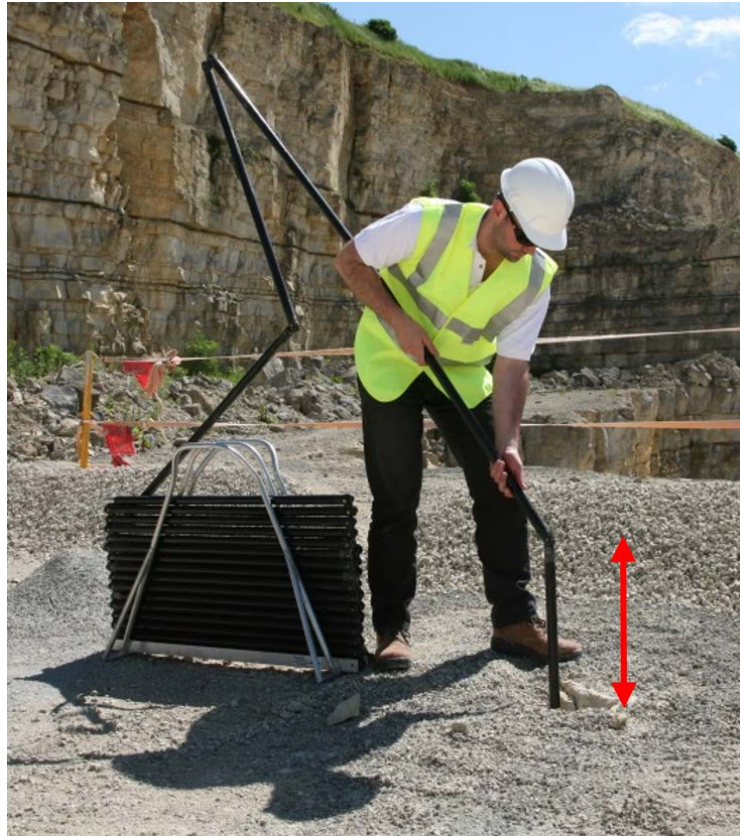
Figure 66 Measuring the rod offset
