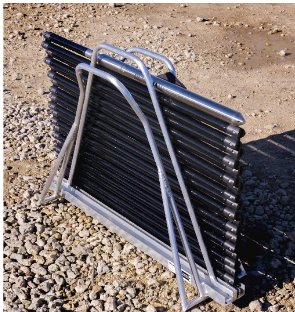
Figure 12 Rod rack with rods and probe attached
