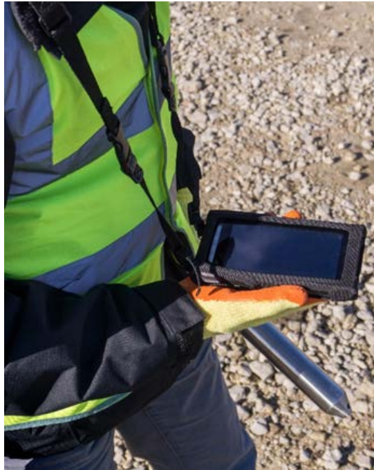
Figure 5 PDA fitted with carry case and neck strap
