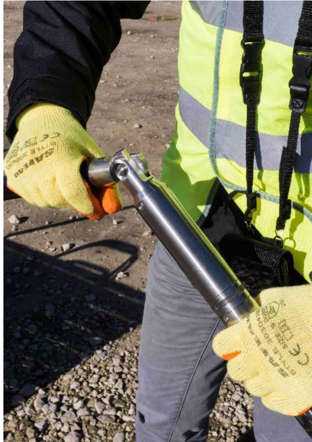
Figure 13 Quick release joint
