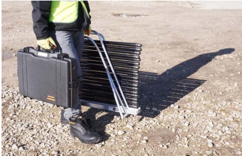
Figure 58 Rodded Boretrak system on-site
