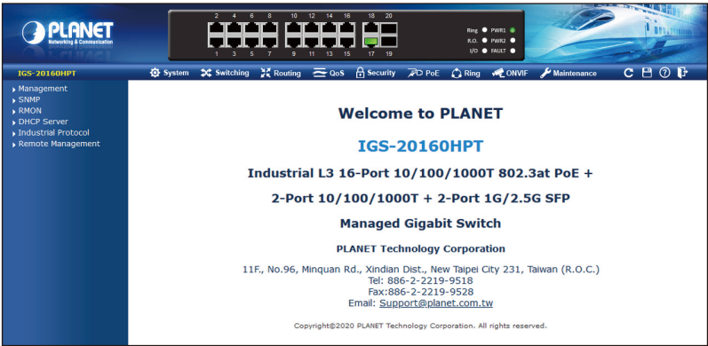
Figure 5-3: Web Main Screen of Industrial Managed PoE+ Switch
