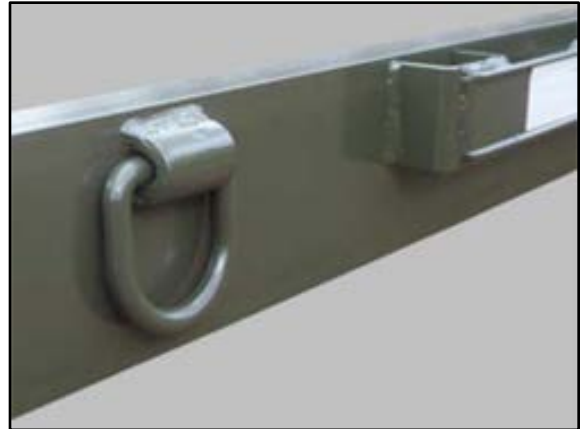
Figure 1-7. "Lashing Ring" Side Rail Mount WLL = 5400 lbs (2449 kgs)
