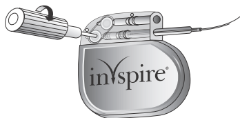
Figure 16. Tighten the lower setscrew
