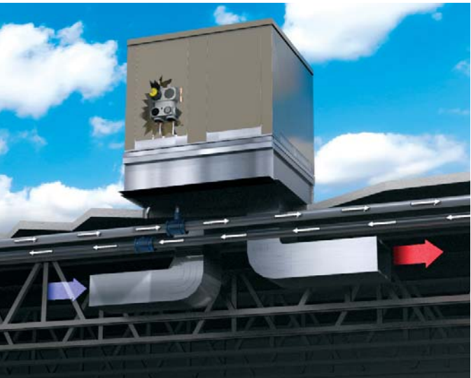
Figure 2: Roof (Curb) Mounted Unit
