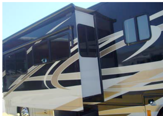
Figure 8-2. Typical Slide-Out Fully Extended
