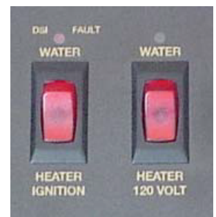
Figure 4-16. Water Heater Switches
