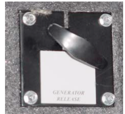
Figure 7-13. Generator “Pull” Cable Slide-Lock Release
