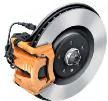
TRW floating caliper brake used on the rear axle
