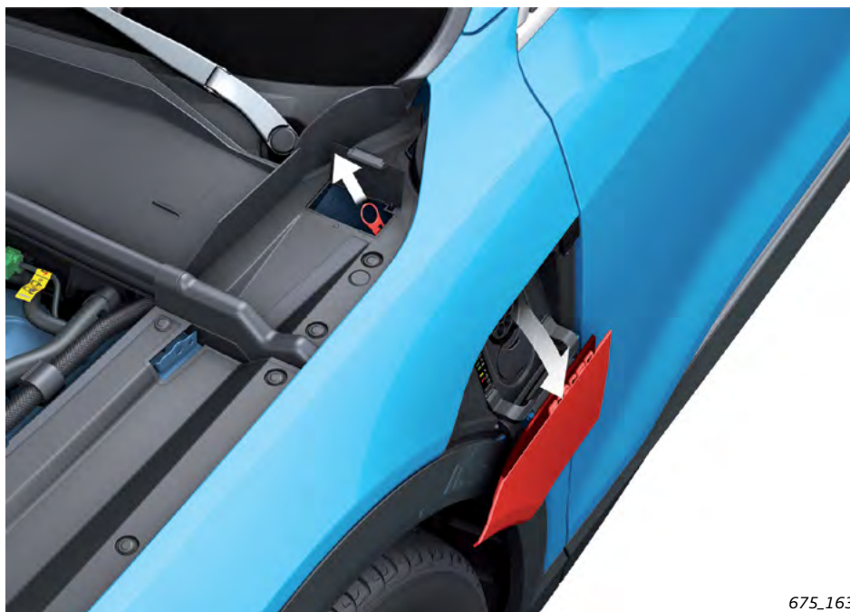
Charging flap manual release
