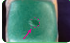
3J 1 cm hole in the Transparent film at the landing-pad relocation site.
