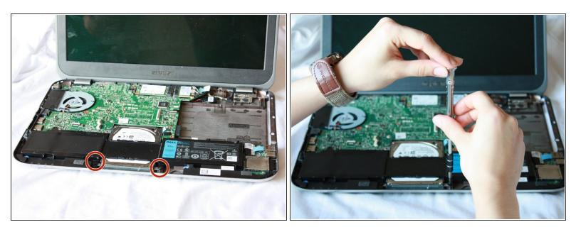
Use a J0 Bit screwdriver to remove the two 6 mm Phillips screws securing the battery located near the bottom of the laptop.
