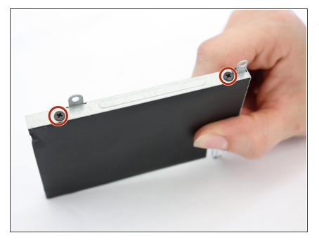
Using a J0 bit tipped screwdriver, remove the four 3 mm black screws on both sides of the hard drive bracket.
