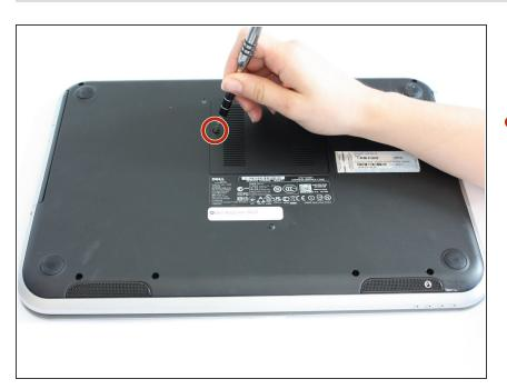
Use a J0 bit tipped screwdriver to unscrew the one 6 mm Phillips screw on the RAM cover.
