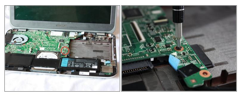
Using a J0 tipped screwdriver remove the 6 mm Phillips head screw located at the center of the laptop on the motherboard.
