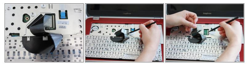
• Flip the little black securing bar near the base of the ribbon with a spudger to release the ribbon from the computer.
