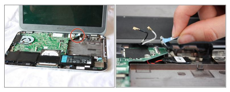
• Gently pull the the blue ribbon upwards to disconnect the computer from the motherboard.
