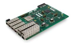
The 1GE/100M/10GE expansion module provides 1GE fanout and 10GE support. The module features 4 SFP and 4 SFP+ ports to enable a combination of 4 100M and 4 1GE ports, or 8 1GE ports, or a combination of 4 1GE ports and 4 10GE ports. As networks evolve, 10GE has become more prevalent, so this internal fanout capability is critical to connect to newer network elements.
