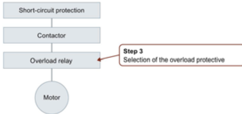
Figure 6-6 Selection of the overload protective device
