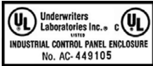
Figure 5-15 Label for a UL-tested empty industrial control panel enclosure
