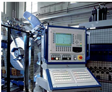
Figure 10-8 Example of operator station with EMERGENCY STOP
