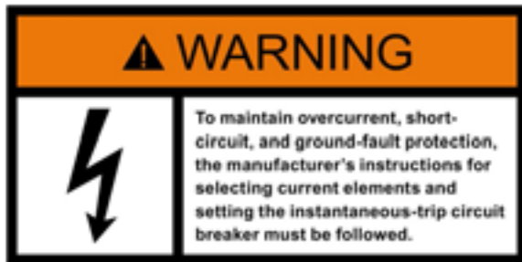
Figure 13-12 Example of warning notice for instantaneous trip circuit breakers
