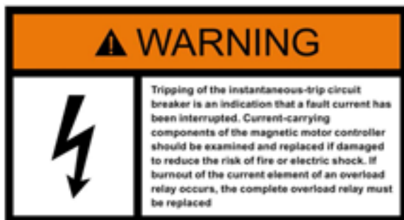
Figure 13-13 Example of warning notice for instantaneous trip circuit breakers
