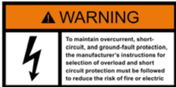
Figure 13-14 Example of warning notice for motor circuit breakers
