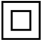
Figure 5-19 "Double Insulation" symbol (protection class 2)
