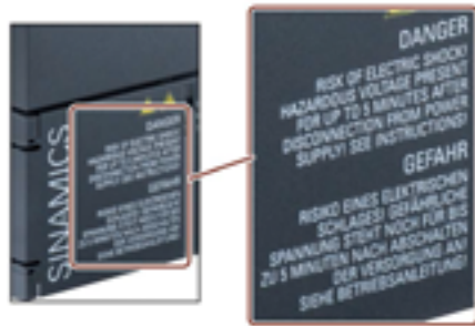
Figure 5-21 Sinamics variable speed drive with warning sign
