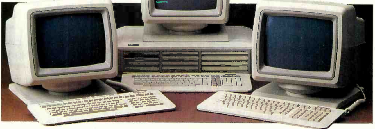
A LAN can join 63 of the pictured MAI 2000 desktop units, each of which can handle 14 users.
