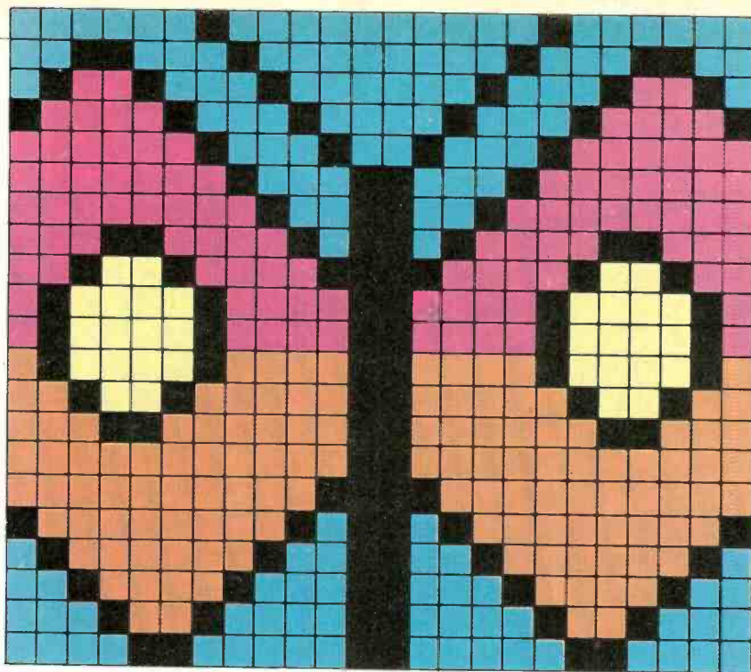
Fig. 1. A simple sprite is plotted on a grid. The bit pattern representing this sprite can then be stored in memory under the name "butterfly."
