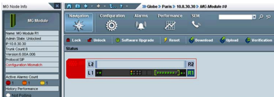
Figure 6-15: Mediant 2000 Information pane Indicating Mismatch
