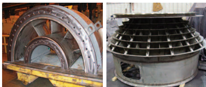
Figure 26. CHROEM 7EA exhaust frame and aft diffuser in latest design configuration.
