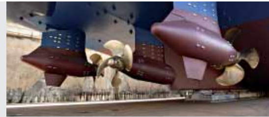
Azipod propulsion systems increase a vessel's efficiency, save fuel and improve maneuverability.
