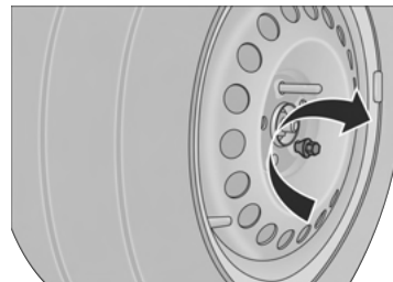
Installing Wheel Bolts
