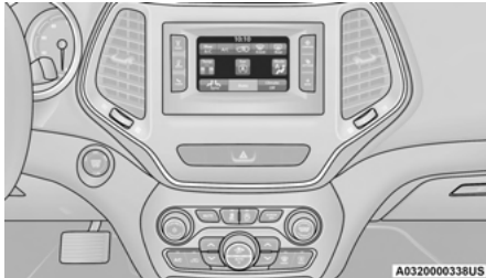
Uconnect 3 With 5-inch Display With Automatic Temperature Controls
