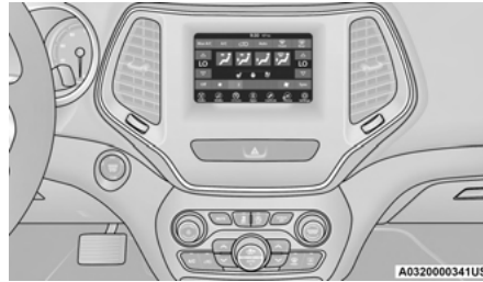
Uconnect 4 With 7-inch Display With Automatic Temperature Controls
