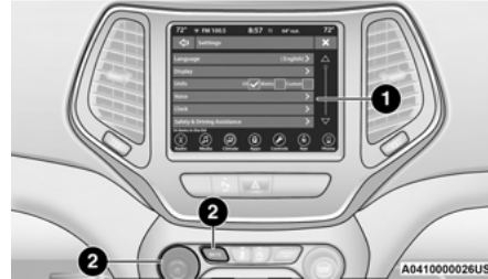
Uconnect 4C/4C NAV With 8.4-inch Display Buttons On Faceplate And Buttons On Touchscreen
