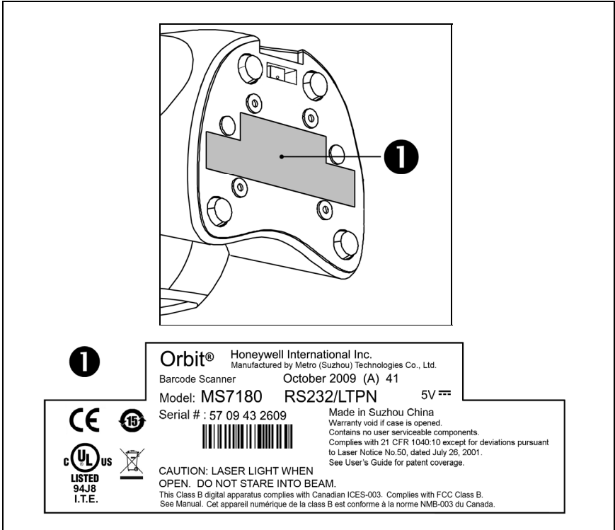
Figure 3. Label Location on the Bottom of the Scanner with Example
