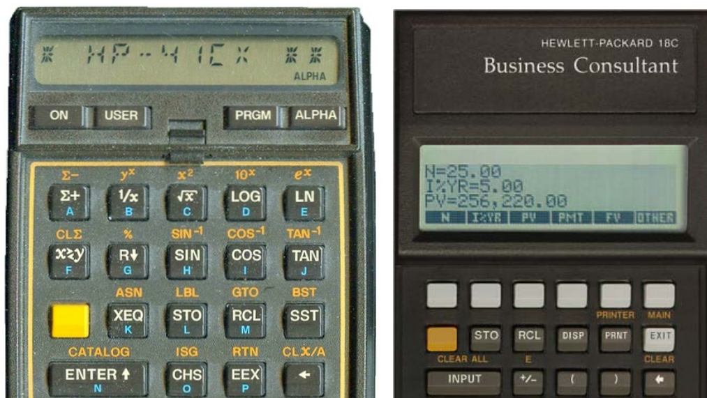
Fig. 2 - The single-line segmented HP41 LCD (left) permitted spelling out function names while the multi-line dot-matrix HP18C screen (right) on the right side of its clamshell case provided a method for labeling a menu of up to six “soft” keys in the top row.
