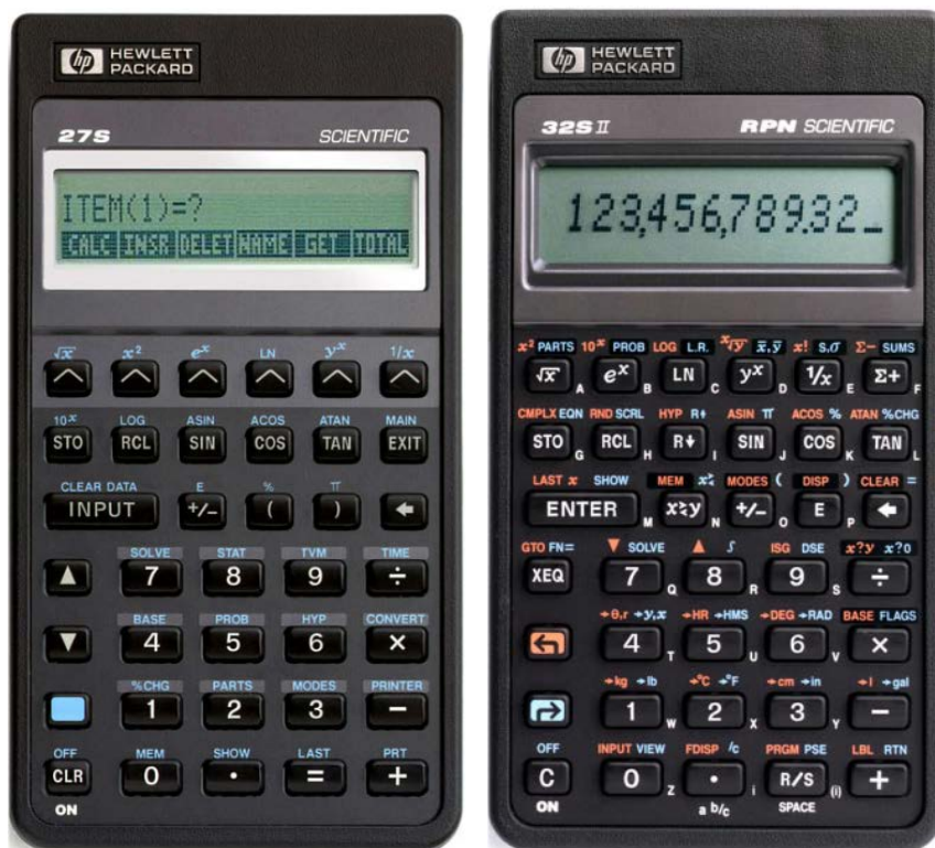
Figure 3. Two Pioneer-series models: the HP27S (left) from 1988, with its clutter value of 1.73 functions per key and HP32SII (right) from 1991, with its second shift key and higher clutter value of 2.73. With their rounded-surface keys, the provision for a function on each key front had been removed.
