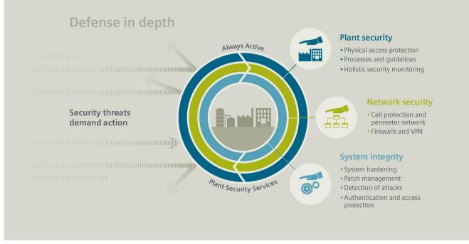
Deep staggered Defense - "Defense in Depth" - as a comprehensive protection concept, according to the recommendations of ISA99 / IEC 62443, the leading standard for security in industrial automation.
