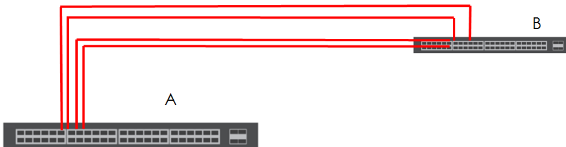
Figure 122 Trunking Example – Physical Connections
