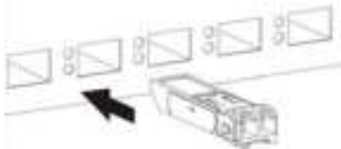
Figure 16 Connecting the Fiber Cables
