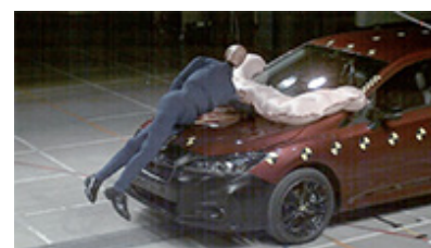
Crash test using a car fitted with the first pedestrian protection airbag in a Japanese-produced vehicle
