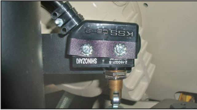
Figure 47. Limit switch (SQ1).
