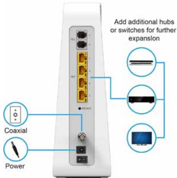
Sample Ethernet to Computer Connection (Connect Box model shown)
