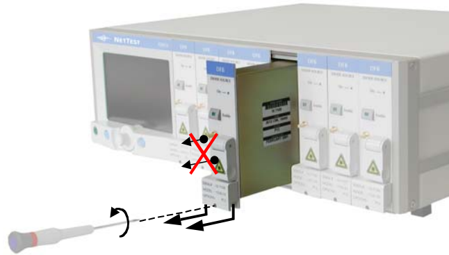
Figure 1-12: How to remove a module from the OSICS mainframe
