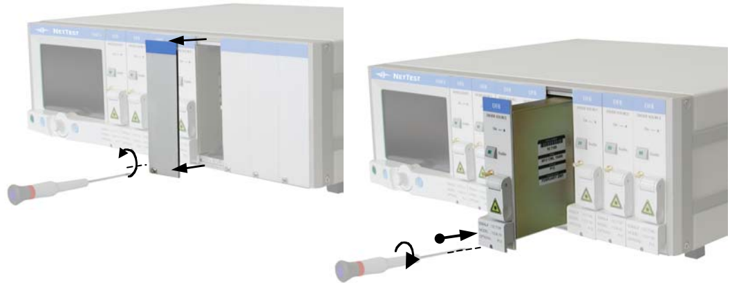
Figure 1-11: How to install a module into the OSICS mainframe
