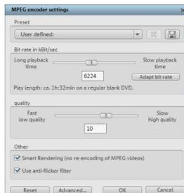
Use the "Encoder" button to access the selection dialog where you can specify the properties of the MPEG encoder (memory requirements, quality, and duration of the MPEG conversion).
