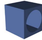
A Without B: This is similar to A subtract B, but it is not a genuine Boolean operation. It cuts holes in object A without capping the holes.
