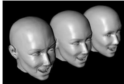
The head rendered with 6,876 triangles, 3,437 triangles and 1,715 triangles.
