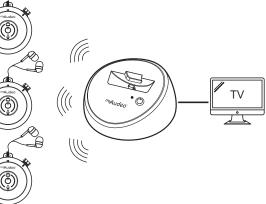
Multiple Receiver Units can be connected to the Base Unit at the same time.
