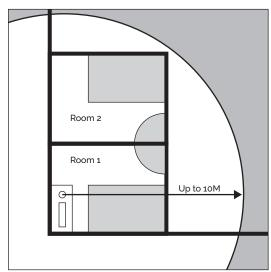
Do not place the transmitter close to metal objects such as shelf bars, reinforced concrete walls etc, as this can decrease the transmitter's range.
