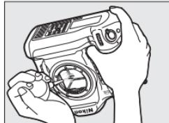
Dirt that can not be removed with a blower can only be removed by Nikon-authorized service personnel. Under no circumstances should you touch or wipe the filter.
