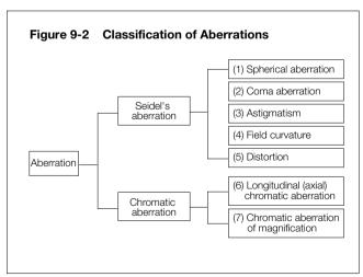
Types (1) to (3) correspond to "expansion of a point image" that goes against requirement (i) for ideal image formation in Figure 9-1. Type (4) corresponds to "curvature of image plane" that goes against requirement (ii) in Figure 9-1. Type (5) corresponds to "deformation" that goes against requirement (iii) in Figure 9-1. Types (6) and (7) correspond to "color blur" of images caused by
