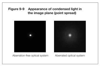
With the proportion of light concentrated in the image plane (intensity of light concentrated in the Airy disk) by an aberration-free optical system serving as 100%, the proportion of light concentrated by an aberrated optical system is known as the Strehl ratio. When graphed, the Strehl ratio reveals peaks in intensity as shown in Fig. 9-10. The higher the SR, the closer an optical system is to being aberration-free.
