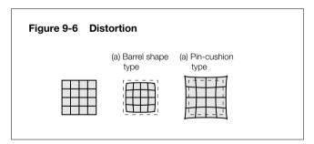
The microscope optical system contains some distortion. When distortion is present, it can bring erroneous results of shape measurements. When a microscope is used for precision measurements, pay close attention to this aberration, for example, by providing it with an aberration compensation function.
