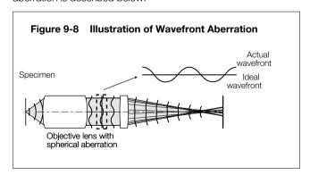
A difference (a degree of disagreement) between the ideal wavefront and the actual wavefront shown above is called "wavefront aberration."
