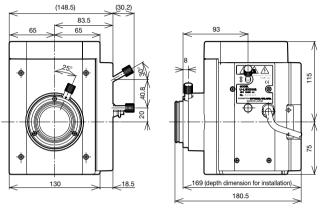
Cable length 2,000mm Accepted lamp: USH-103OL Weight: 2.7kg
