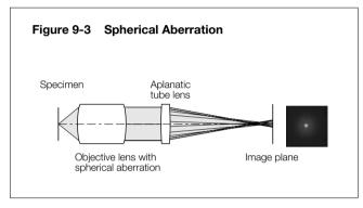
It is said that objective lenses with larger N.A. have better resolution but worsen spherical aberration. Our advanced design and manufacturing techniques have realized good optical performance even with large numerical aperture.
