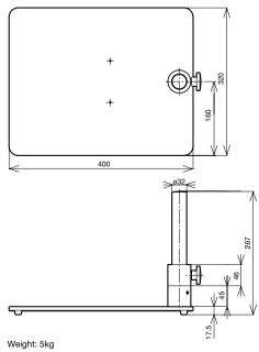
Weight: 1.8kg Weight: 5kg Unit: mm
