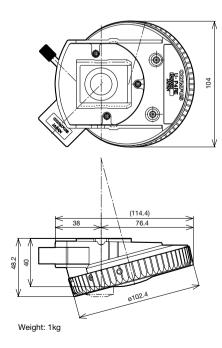
U-P6RE Centerable sextuple revolving nosepiece with slider slot for DIC
