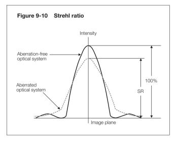
A Strehl ratio of 80% is typically called the diffraction limit, and lenses with a lower ratio lack the performance required to serve as an objective lens. A ratio of over 95% means that the lens' performance in general observations is comparable to that of an aplanatic lens (which is corrected for spherical aberrations and coma).
