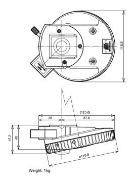
Insert the DIC dummy when not using the DIC slider
