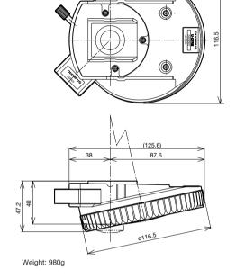
U-P4RE Centerable quadruple revolving nosepiece with slider slot for DIC
