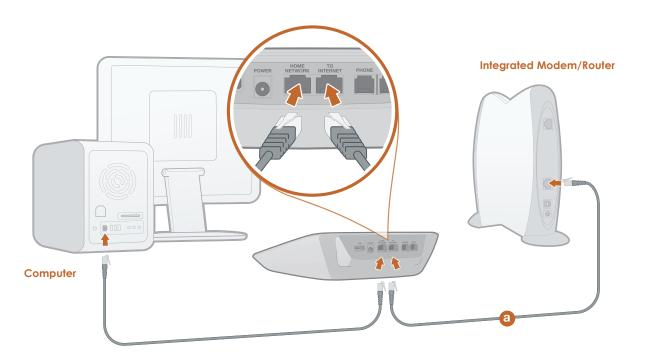
Connect your computer to Ooma Telo (optional) If your computer is connected directly to your router, disconnect the end plugged into the router and plug it into the HOME NETWORK port. This allows Ooma to prioritize your phone calls.
