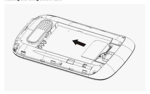
Metal contact surface of SIM card is easily scratched. You must take out SIM care carefully before the assembly. Power off the phone, remove the rear cover, battery or other external power supply.
