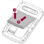
Warning: Make sure to power off the phone before taking out SIM card, battery, otherwise your SIM card might be damaged.
