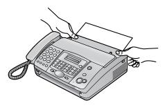
**6** For KX-FT902: Press [FAX/START], then tear off the excess paper by pulling it towards you.
