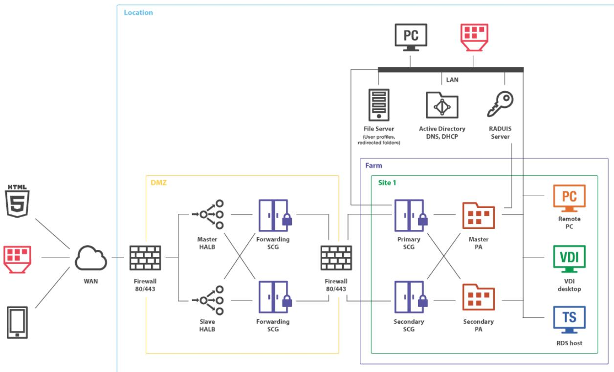
In a configuration of this type the second-level authentication via a RADIUS server is performed first. If the authentication procedure is successful, the next authentication takes place at the Active Directory level using either a user name and password or a smart card.
