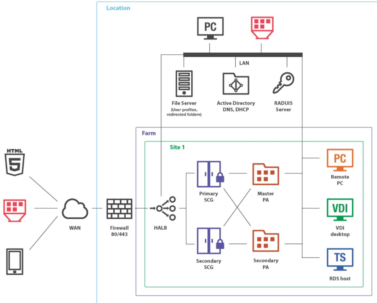
\*300 users through SSL tunneled gateway mode or 500 standard gateway connections, assuming the gateway machine is only acting as such (with no other demanding services using these machines).
