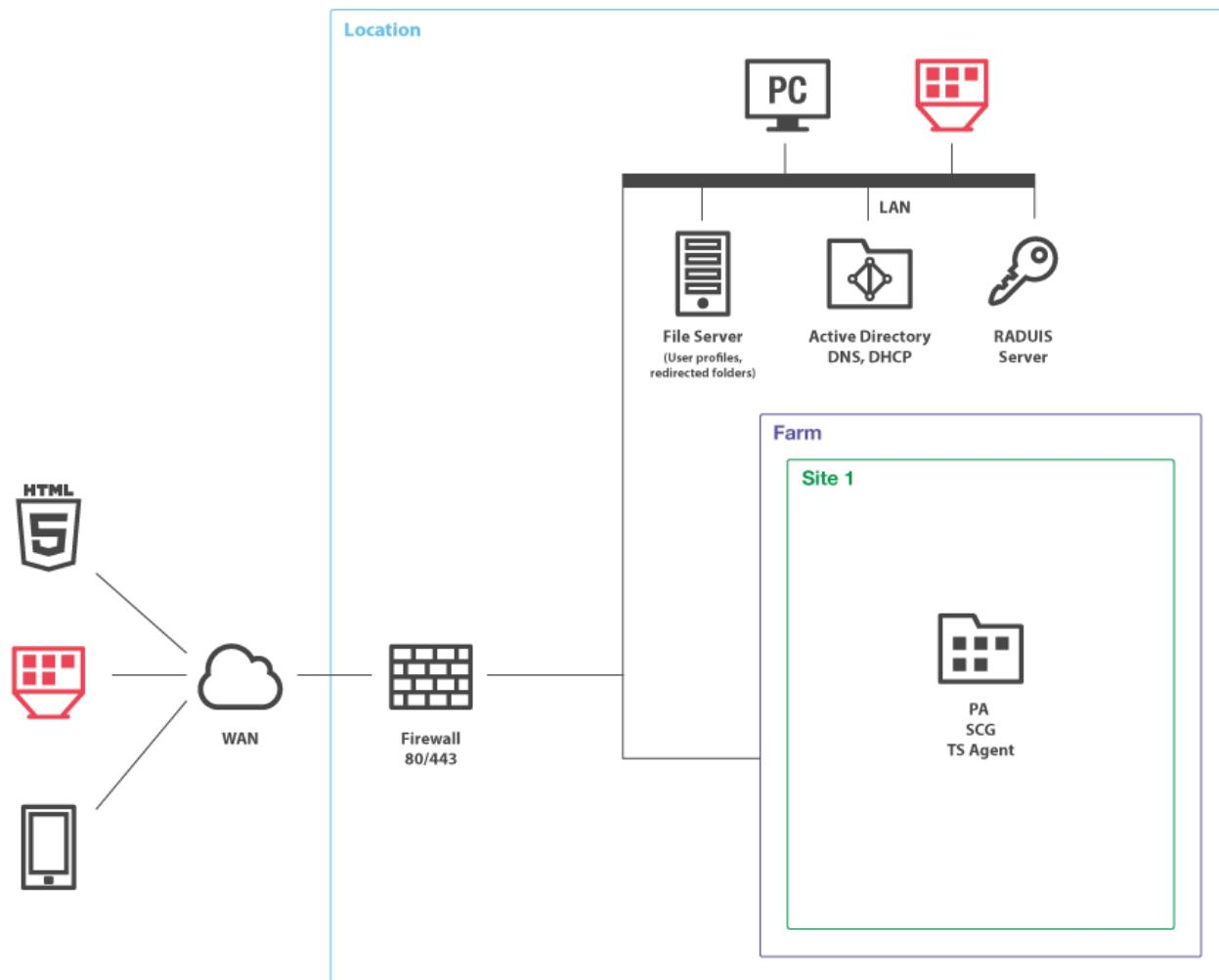
The left side of the diagram displays client devices that can connect to Parallels Remote Application Server. In the example above, the clients are (from top to bottom):
