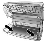
9 Break the chip card from the Plug'n'Print card. Insert the chip card in the plug socket on the left hand side next to the ink film tray.
