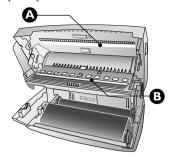
5 Clean the feed roller (A) and the underside of the support pad of the feeder roller (B) with a soft, lint-free cloth moistened with cleaning alcohol (96 percent). Rotate the feed roller; You must clean the entire roller.
