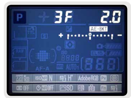
AEB settings on a Nikon D7000 (3 frames, at +/- 2 EV)
