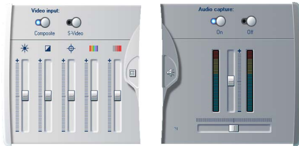
Video (L) and audio (R) panels for setting levels during analog capture.
