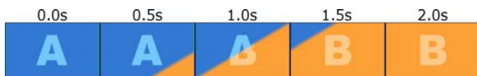
Diagram: Five snapshots from the life of a 2-second diagonal wipe transition.
