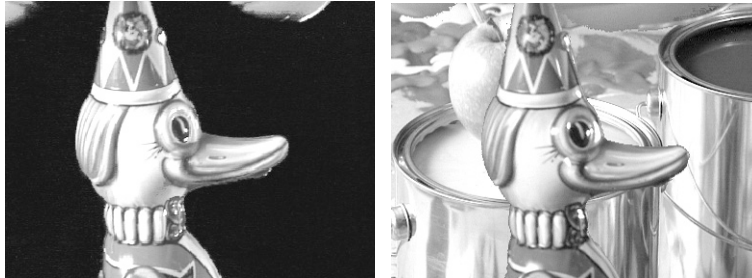
Luminance Key: a different image signal is superimposed over areas with the same luminance
