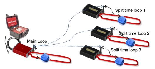
Note that the LoopBox has an internal buffer for 1000 detections. Even if the connection between LoopBox and Active Extension is interrupted, the detections will not be lost: once the connection recovered, the LoopBox will transmit the buffered detections. Thanks to the precise internal clock of the LoopBox, the detection time will still be correct and precise.
